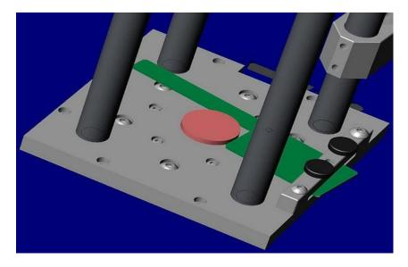
This fixture also eliminates the problem of type III samples *migrating* with the application of the contact pressure when oil or grease is used for surface-contact-resistance abatement.
